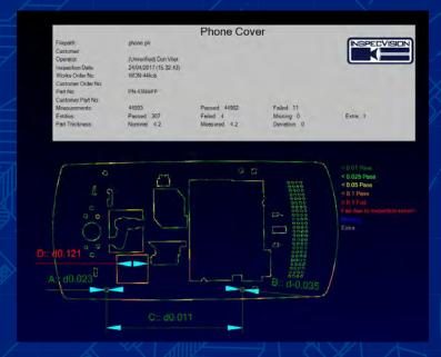
Figure 3: 2D Inspection with Deviation Map
