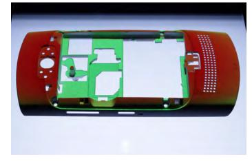
Figure 5: Projected Augmented Reality Deviations
