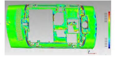
Figure 6: Comparisons to 3D CAD Model
